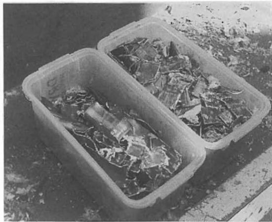
Fig.30 Shreddered Channel Box
